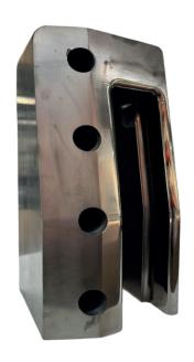
Capa nitrurada: 85 µm Dureza 1200 HV (DIN 50190-3)
